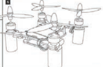
Attach the battery and motor to the frame. Attach the propellers to the motor.
